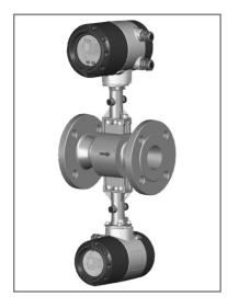
This is a genuine redundant system with two independent measuring sensors and two signal converters. This provides twofold functional reliability and availability of the measurement. This variant is ideally suited for measurements in multi-product pipelines. In such pipelines, two different products are moved through one after the other. One signal converter can be programmed for one product, and the other signal converter
