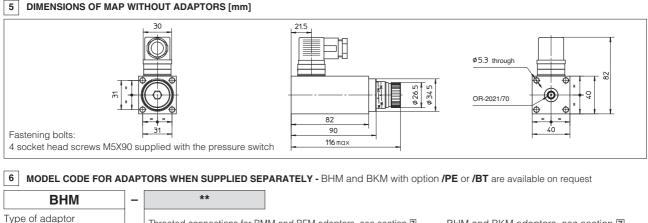
Threated connections for BMM and BFM adaptors, see section 2 BHM and BKM adaptors, see section 7 BMM = male BMF = female **BFM** = in-line 06 = G 1/4" (BMM, BMF, BFM) 20 = G 3/4" (BFM) **11** = port P **12** = port A and B **13** = port A **14** = port B **17** = port P and A **18** = port P and B **10** = G 3/8" (BMM, BFM) **15** = G 1/2" (BMM, BFM) BHM = ISO 4401 size 06 (BMM, BFM) **25** = G 1" (BFM) BKM = ISO 4401 size 10 32 = G 1 1/4"(BFM)
