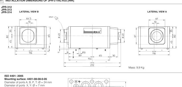
Diameter of ports A, B, P, T:  $\emptyset$  = 24 mm Diameter of ports X, Y:  $\emptyset$  = 7 mm Seals: 4 OR 4112; 2 OR 3056
