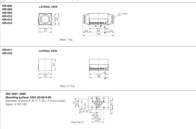
Fastening bolts: no 4 socket head screws M5. The lenght depends on number and type of modular elements associated.
