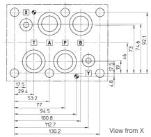
Fastening bolts: no 6 socket head screws M12. The length depends on number and type of modular elements associated.
